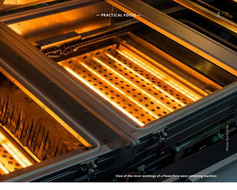
been achieved: The risk of dirt build-up has been reduced and inerting is now possible regardless of its extent. This allows the ROL value to be stabilised and dross to be significantly reduced. Furthermore, nitrogen consumption can also be reduced, but here the condition of the unit plays a part.
