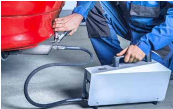
Car exhaust emission testing
