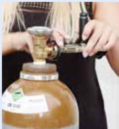
Ensure cylinder is standing securely, unscrew cylinder cap if applicable. Screw inflation valve on to cylinder valve by hand (do not use a tool!)
