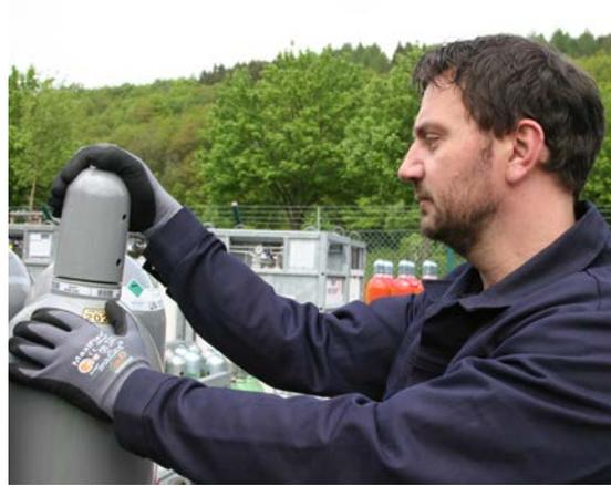
**and have a thorough examination of the gas cylinder carried out.** Never conceal or fail to mention damage to a gas cylinder. This would endanger your own safety and the safety of others, and it could have legal consequences.
