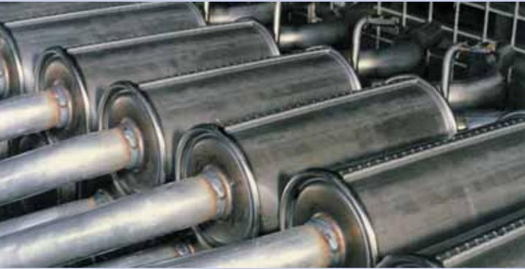
*Above: The welded seams on an exhaust system can be clearly seen.*
