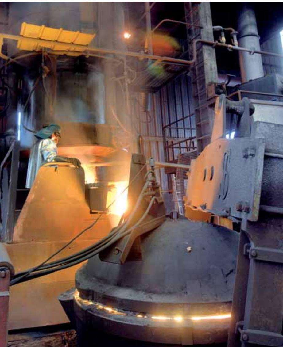
*Perfect control: coke consumption can be reduced by injecting oxygen into the cupola.*
