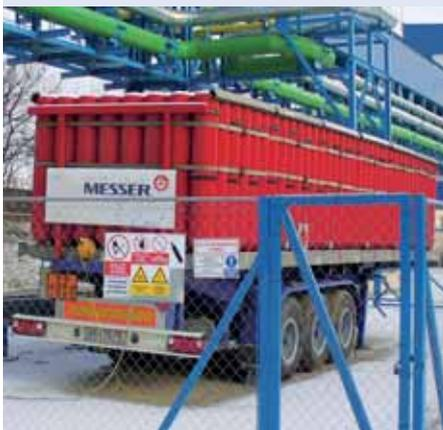
Hydrogen is supplied to U.S. Steel in battery trucks like this.
