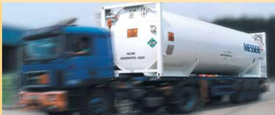
*The liquid helium is transported from source to filling plant in special tank containers.*
