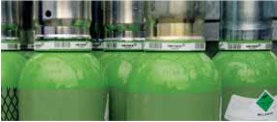
Every step of the supply chain can now be tracked thanks to the bar code labels on the gas cylinders.
