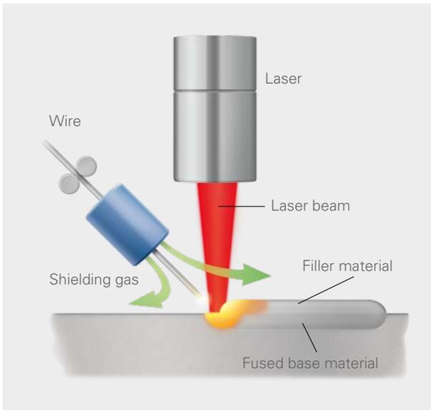
Laser deposition welding with wire
