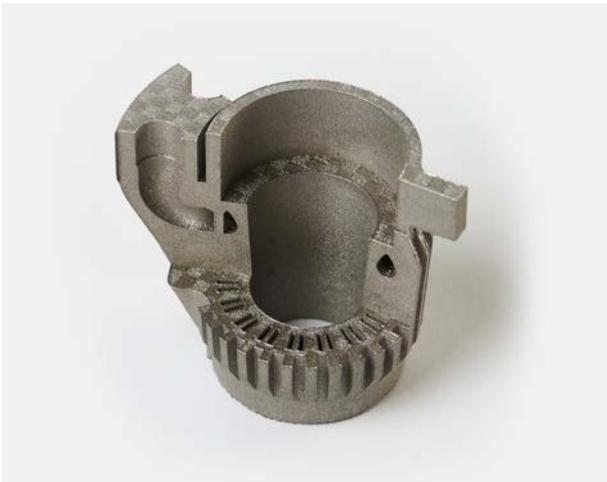
Cooled welding nozzle made of CrNi steel, developed by ifw Jena
