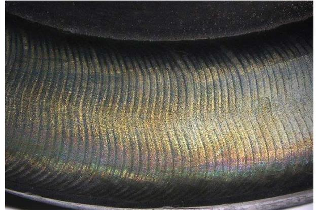
Plasma-arc deposition welding
