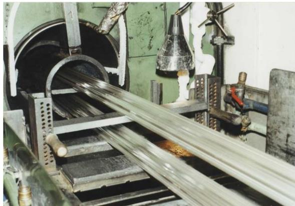
*Figure 1: Extrusion*
