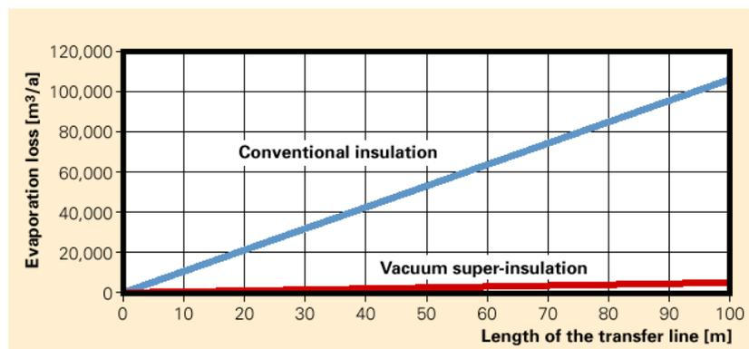
Figure 8: Evaporation in supply line
