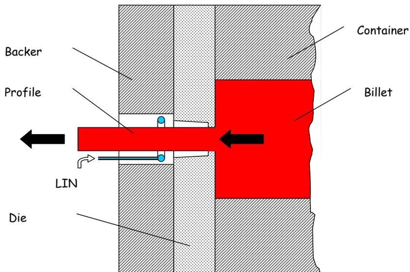
Figure 3.1: Ring nozzle cooling
