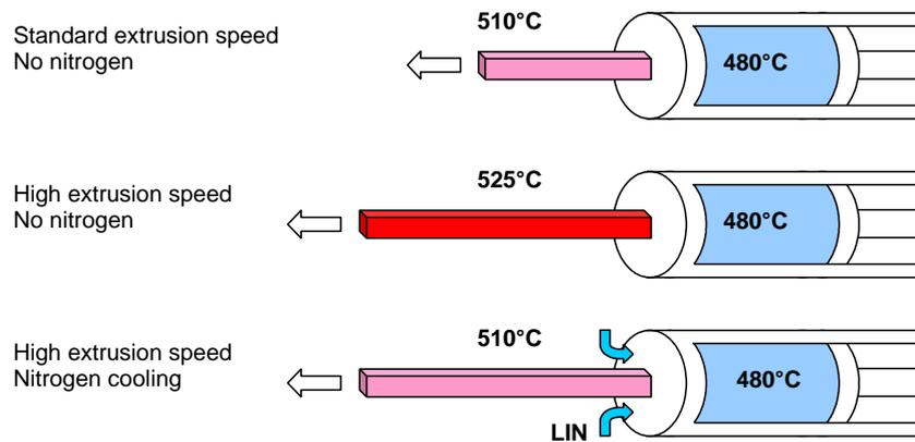
Figure 5 increased extrusion speed
