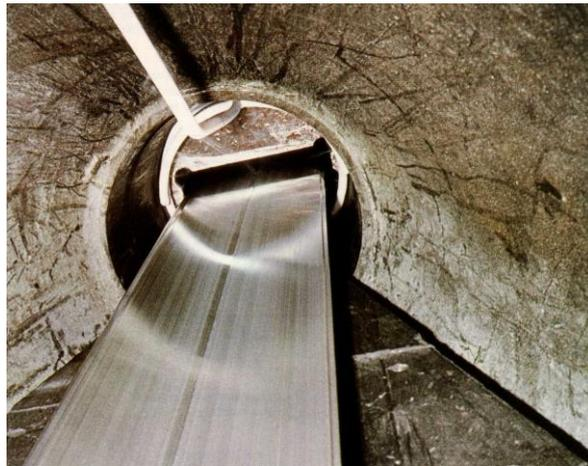
Figure 3.2: Ring nozzle cooling
