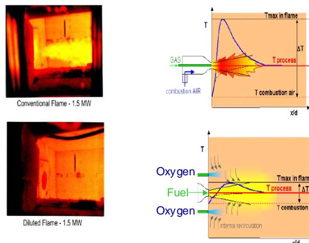
Figure 3: Diluted combustion – a possibility to reduce NO<sub>x</sub> [3]
