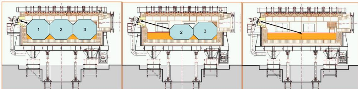
Figure 4: Development of the changing of distance between scrap metal and the burner mouth in a hearth-type furnace<sup>[5]</sup>.
