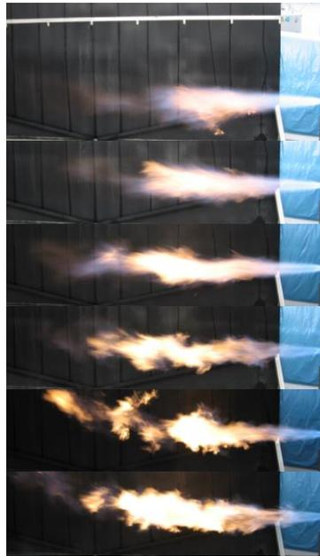
*Figure 5: Flexible Flame of a 900 kW Oxipyr®-Flex burner from 1 m to 3 m and from a hard to a soft flame at the free test stand*
