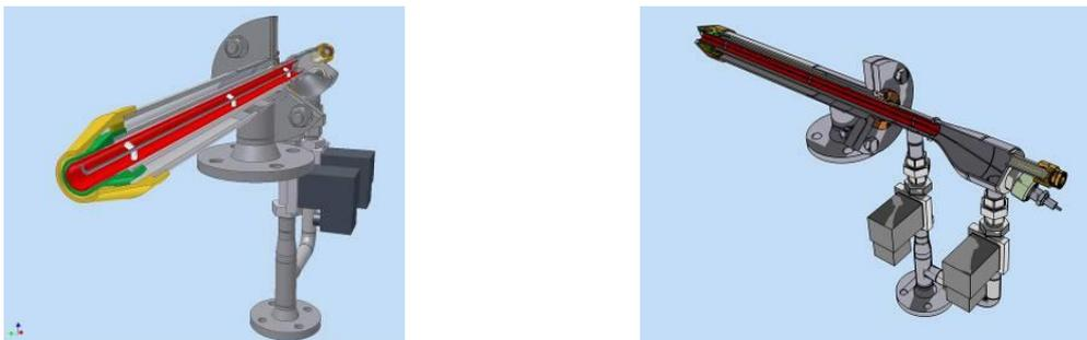
*Figure 6: Design of a 900 kW Oxipyr®-Flex for short drum furnace for lead recycling*
