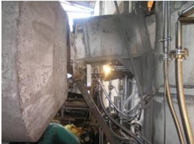
*Figure 8: Burner under offgas system*
