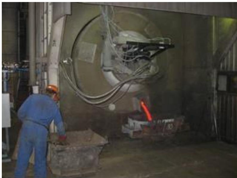
*Figure 7: Burner opposite the offgas system*
