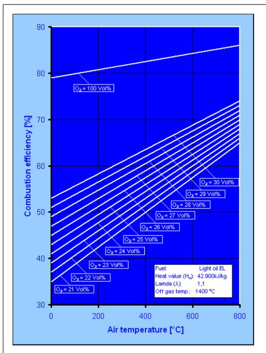
Figure 1: Influence of the combustion air temperature and the oxygen concentration on the combustion efficiency<sup>[1]</sup>
