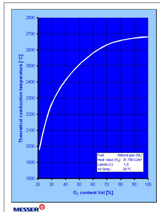
Figure 2: Theoretical flame temperature for the stoichiometrical combustion of natural gas as function of the oxygen content<sup>[1]</sup>
