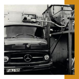
Some food has to be kept cold on its way to the customer, and that was also true in the past. A predecessor of today's EcoLIN vehicles was used for this purpose. It still cooled the load directly, however, which required refilling with liquid nitrogen.
