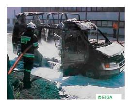
Acetylene gas leaking from the valve of a gas cylinder ignited inside a delivery van. The driver narrowly escaped. The vehicle burned out in just two minutes.
