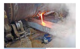
Oxypyr–Plon burner for oxygen dosing in frit production
