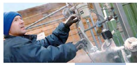
The volume of liquid nitrogen can b controlled precisely during cement cooling.
