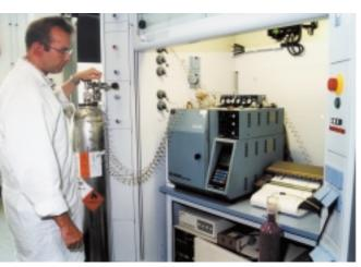
Calibration gas test on the gas chromatograph at the special gases plant in Krefeld-Gellep
