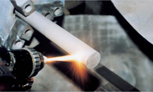
...flame spraying (left) and manual WIG welding...
