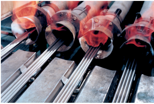
Tempering of special wire in a tubular wire drawing furnace
