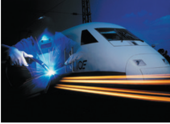
MIG welding of aluminum in rail vehicle construction.
