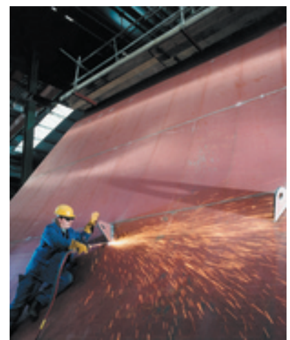
Acetylene flame cutting in shipbuilding.
