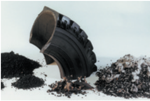
Rubber granulate from old tires: Elastic materials – not just rubber – are easier to grind at low temperatures
