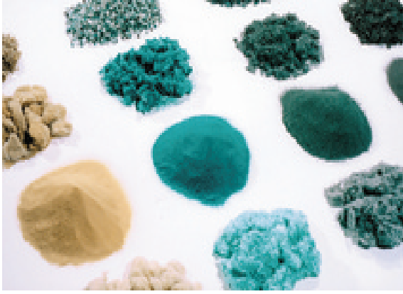
Fine plastic powders through cryogenic milling separation
