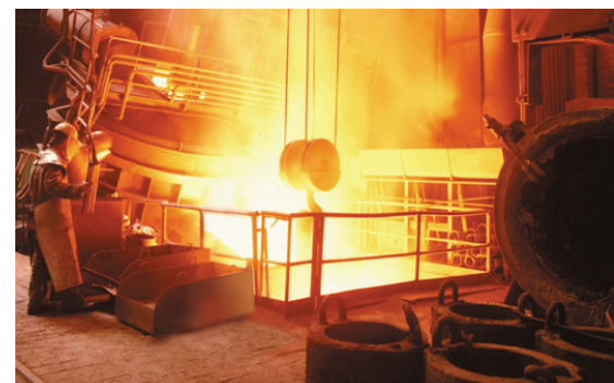
Tapping a steel melt from an electric arc furnace.
