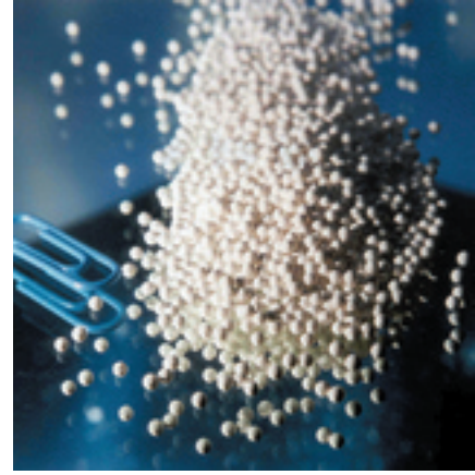
Fine pellets from chemical melts thanks to nitrogen
