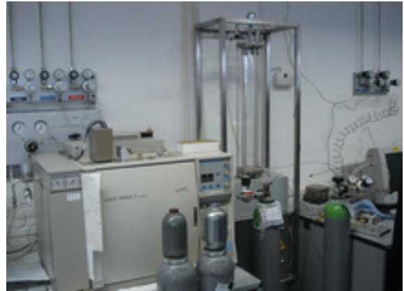
FT-IR spectrometer with long-path cell
