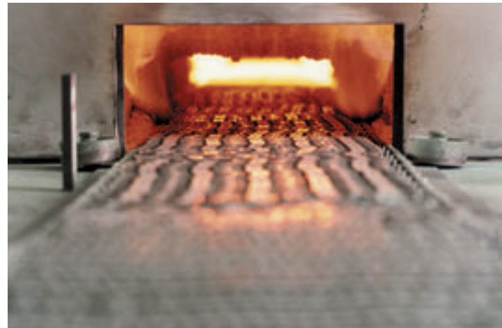
Figure 4: Sintering in conveyor furnace
