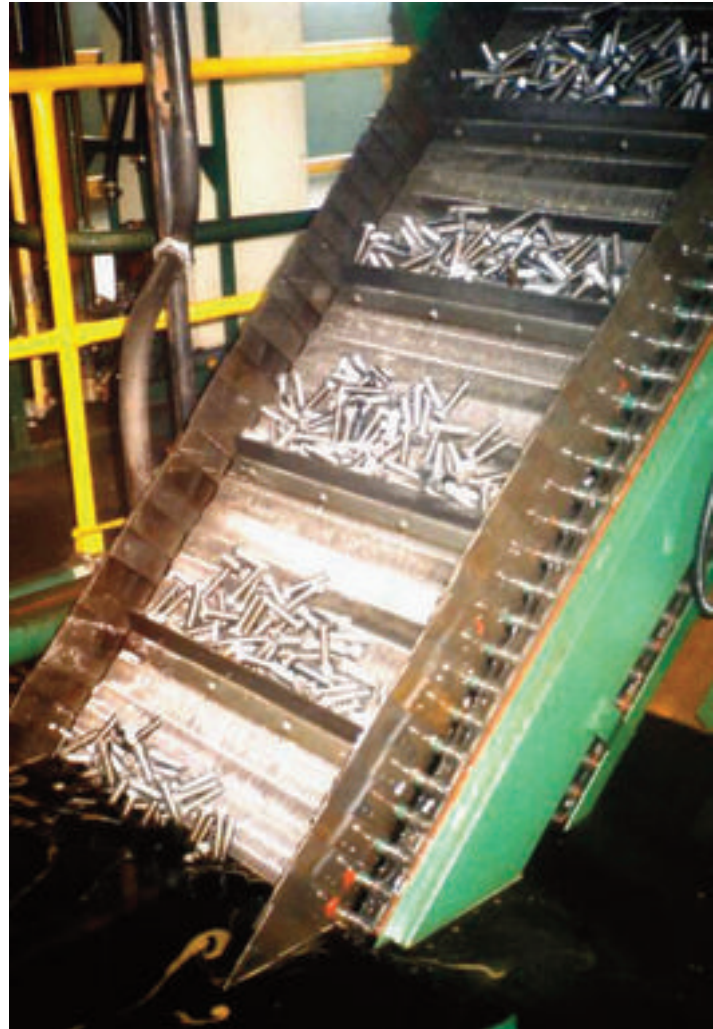
Fig. 7: Hardened screws leave the oil bath.
