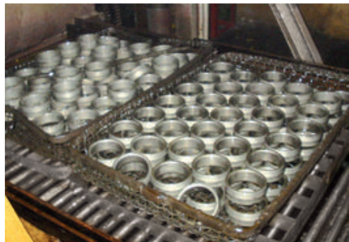
Fig. 5: Annealed bearing rings of 100 Cr6 steel
