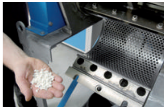
Pre-crushing with cryogenic cutting mill
