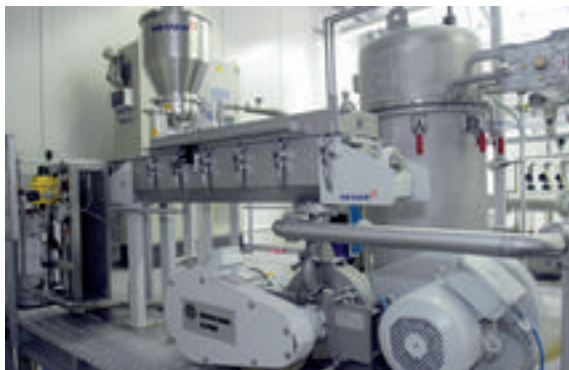
Cryogenic grinding with pin mill
