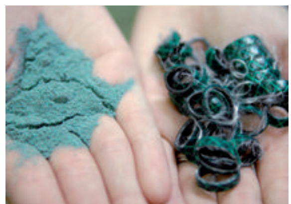
PVC hoses before and after cold grinding
